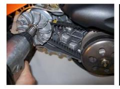
Clean the transmission area with compressed air.
