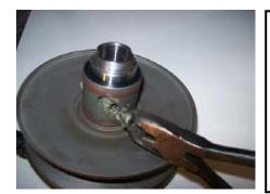
Remove guide pins using pliers. Use caution as marring or gouging the pins will cause excessive wear.
