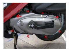
Remove the bolts retaining the transmission cover.
